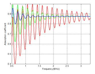
Fig. 2 – Absorption coefficient curves of backing material for different loss factor of base material (red line:0.05, green line:0.1, blue line:0.2)
