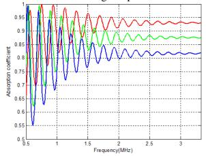
*Fig. 1 – Absorption coefficient curves of backing material for different volume content of tungsten powder (red line:20%, green line:30%, blue line:40%)*
