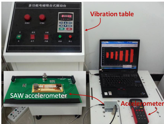
Figure 8. The measurement set-up of the SAW acceleration sensor.
